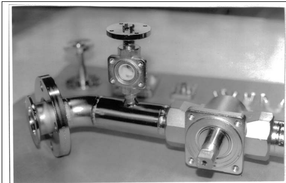
FIGURE 4 ELECTROPOLISHED MANIFOLD FOR HIGH PURITY PROCESS
